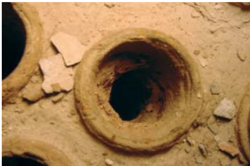
Sludge deposits in tubes.
