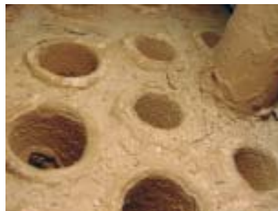
Sludge deposits in tubes.
